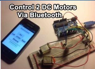
A photograph showing a smartphone displaying an app interface, connected via Bluetooth to an Arduino board which is controlling two DC motors on a breadboard. | View Project on Random Nerd Tutorials | Click <a href="#">here</a> |
